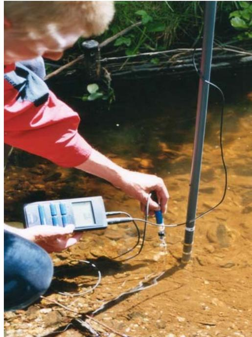
*Fig. 2: Device for measuring redox potentials in defined sediment depths*
