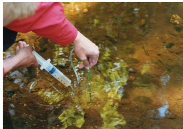
*Fig. 3: Method of sampling fixed volumes of interstitial water from defined sediment depths*
