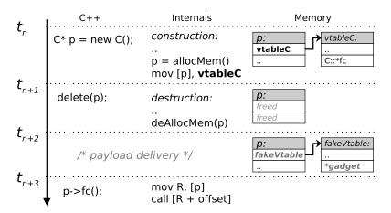
**Figure 3:** The C++ stages, internal low-level operations, and resulting instance's memory layout of a use-after-free exploitation process utilizing vtable hijacking
