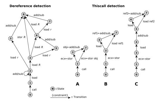
Figure 6: State machines used to detect consecutive dereferences and this call in virtual dispatches. Transitions may be constraint (by e.g.: mnemonic: add, source: add v, destination:  $v \leftarrow add$ )
