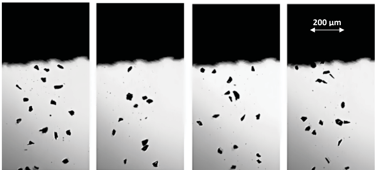
Figure 8: Particle distribution in abrasive air jet
