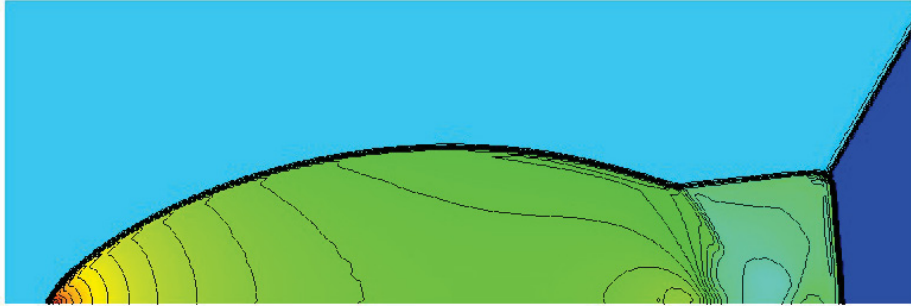
Figure 5: Double Mach reflection problem: (a) density and (b) pressure distribution at T = 0.2 . Discretization: synchronized FCT algorithm, 65,536 Q_1 elements, \Delta t = 10^{-4} .
