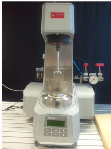
Figure 4.1: The Physica MCR 301 rheometer with plate-plate device
