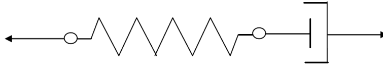
Figure 2.7: Rheological model for viscoelasticity.
