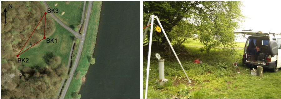
Figure 1.2: Field test location, Kemnader See, Bochum, Germany: (left) configuration of boreholes BK1-BK3. Pumping operations are performed in one borehole and pressure is monitored at all three wells. Interpretation and inversion of information recorded at the boreholes allows for characterization of the material surrounding the wells (source: Google Earth, modified with lines); (right) borehole inspection with different sensors to characterize the rock surrounding the well.
