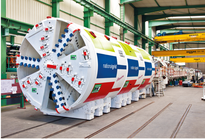
Figure 2.2: Earth Pressure Balance (EPB) shield TBM used in London. The diameter of the cutter head is 4.7 m. (Copyright: www.herrenknecht.com )
