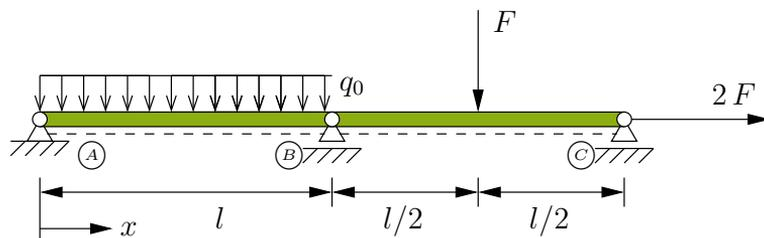
**Geg:**  $l, F, q_0 = F/l$     **Lsg:**  $M(x = l) = q_0 l^2/8, M(x = 3l) = F l/4$
