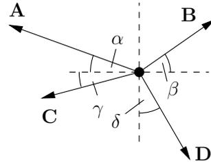
**Geg:**  $A = 1500 \text{ N}$ ,  $B = 1000 \text{ N}$ ,  $C = 1200 \text{ N}$ ,  $\alpha = 20^\circ$ ,  $\beta = 35^\circ$ ,  $\gamma = 15^\circ$
