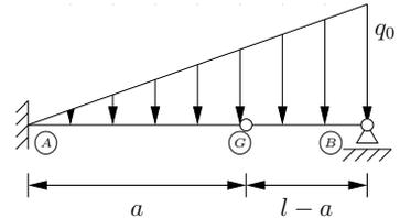
$$\text{Lsg: } A_V = \frac{q_0}{6l} (a^2 + al + l^2), \quad M_A = -\frac{1}{6} q_0 a (a+l), \quad G_V = -\frac{1}{3} \frac{(l-a)(a + \frac{l}{2})}{l},$$
