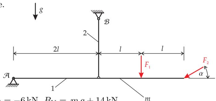
**Lsg:**  $A_H = 4\sqrt{3} \text{ kN}$ ,  $A_V = -6 \text{ kN}$ ,  $B_V = mg + 14 \text{ kN}$
