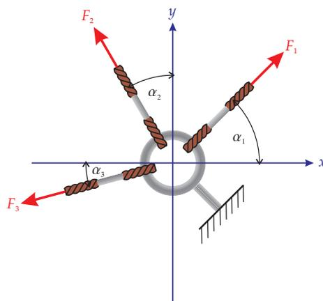
**Geg:**  $F_1 = 100 \text{ N}, F_2 = 150 \text{ N}, F_3 = 250 \text{ N}, \alpha_1 = 45^\circ, \alpha_2 = 30^\circ, \alpha_3 = 15^\circ$
