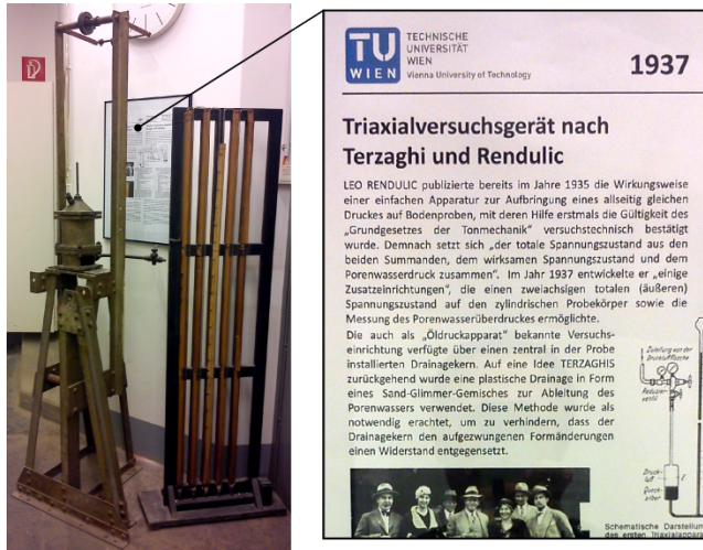
Figure 2.2: Historical devices in the laboratory founded by Karl v. Terzaghi at Vienna University of Technology in 1929: Worldwide, the first triaxial apparatus for pore water pressure measurement. Pictures taken at the Institute for Geotechnics and published with permission of Em. O. Univ.-Prof. Dipl.-Ing. Dr. techn. Dr. h.c. mult. Heinz Brandl, TU Vienna, Austria.
