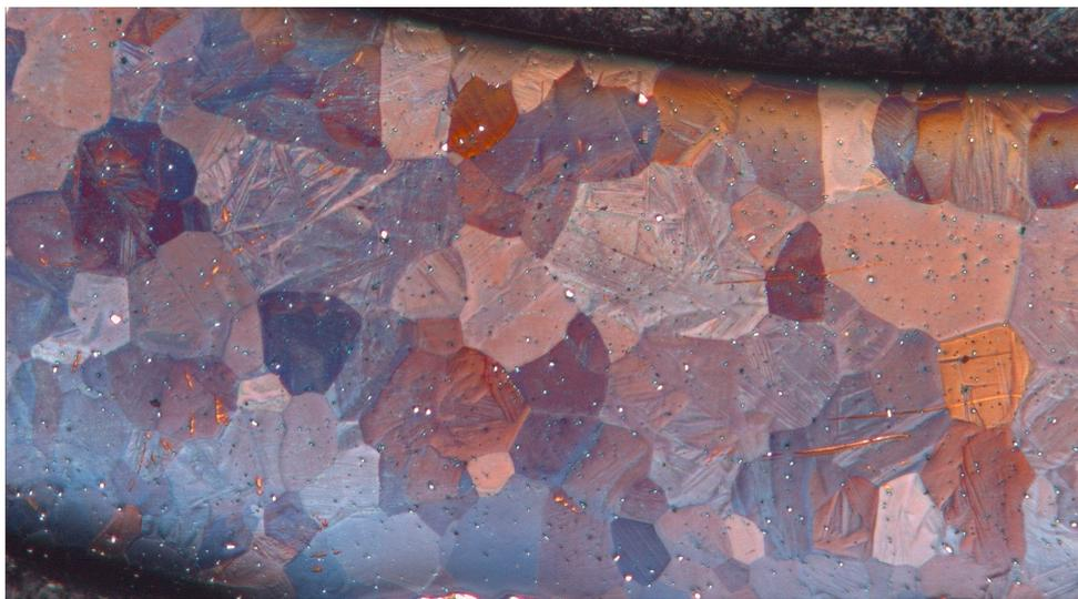
Figure 5.4: Polished micrograph section of the wall within the gage section, magnification of 100x
