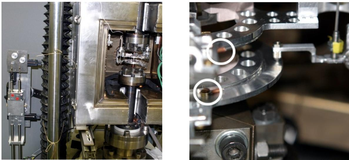
(a) General view of the strain measuring device, outside the temperature chamber on the left: deflection rollers and inductive transducer system for the twist measuring
