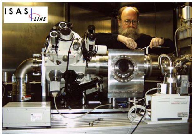
Figure 1. ISAS prototype spectrometer for synchrotron radiation induced wavelength X-ray fluorescence spectrometry.
