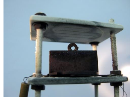
Figure 3: Heating elements and sample holder with sample [4]
