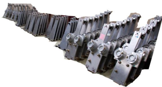
Figure 1: Alignment plates before installation.
