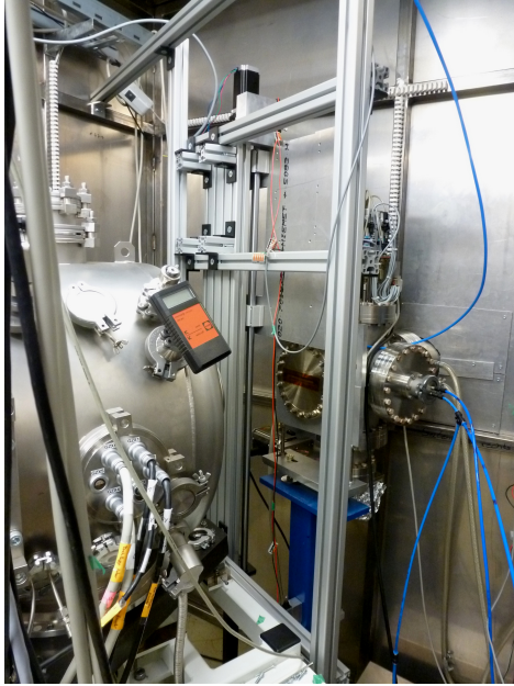
Figure 1: New deep x-ray lithography setup at BL1 of DELTA. Left: photograph[1]; Right: construction drawing
