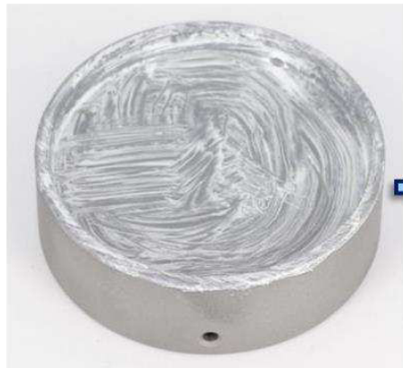
GJS-400-15 sandgestrahlt + Bornitrid
