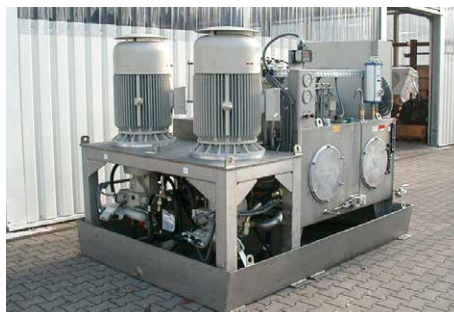
Hydraulic power unit for lock systems, complete stainless steel model, with a backup diesel engine.
