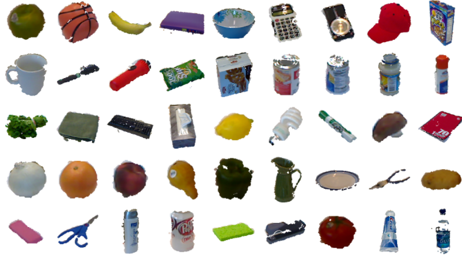
Figure 7.6: RGB-D Object Dataset [45] from the Faculty of Computer Science and Engineering at the University of Washington. The dataset contains 300 objects in 51 categories provided as segmented point clouds and masked depth images.
