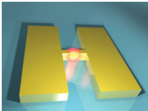
Theoretically proposed gold nano-antenna with maximized central field enhancement
