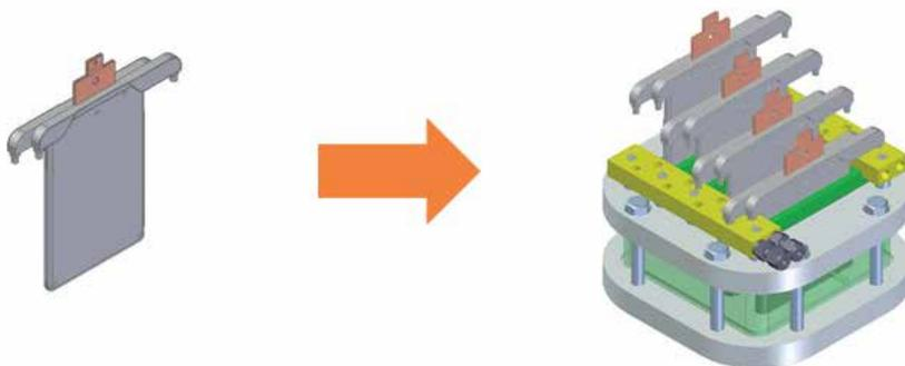
Fig. 1: Schematic drawing of the modularly constructed electrolyser with four individual cells.
