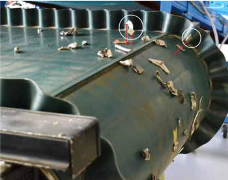
Fig. 1: Separating rare earth magnets with eddy current separators
