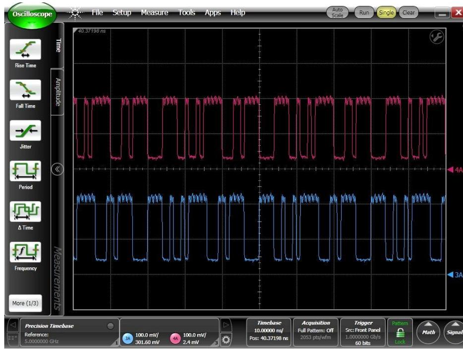
Fig. 3-40 Measured results of the digital baseband test-chip showing two selected outputs generating the same output bit sequence. The results correspond exactly with the expected bit sequence on the two outputs.
