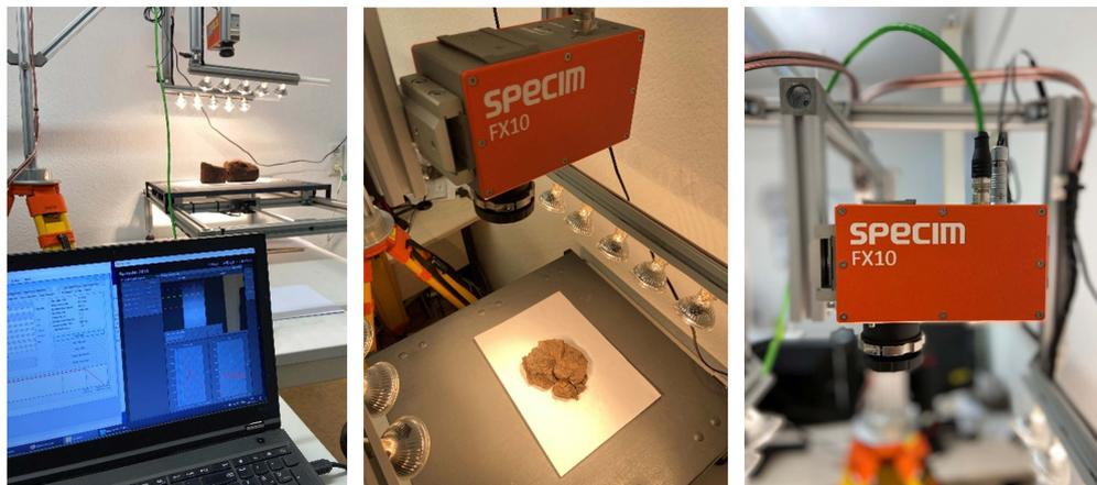
**Fig. 5.** Experimental set-up for hyperspectral scanning of Schleenhain and Peres samples in TRIM4Post-Mining EU Project. Source: THGA
