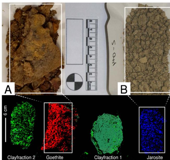
**Fig. 6.** Spectral mapping using supervised classification from Litov AMD in the Sokolov lignite region. Modified from [30].
