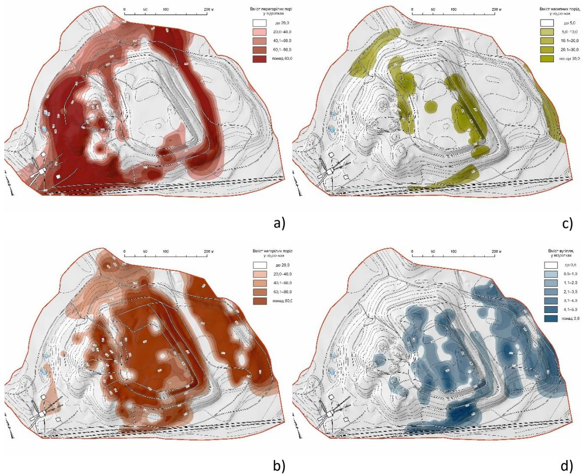
**Fig. 2.** The composition of lithological deposits within the rock dump of the “Vizeyska” mine: a) content of burnt rocks; b) content of unburnt rocks; c) bulk rock content; d) coal content
