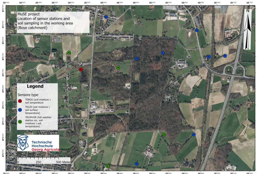
Fig. 8. Position of MuSE soil- and weather sensors.
