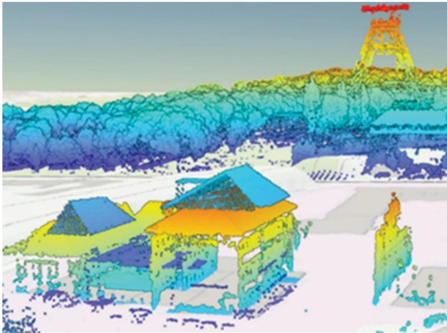
**Fig. 4.** Example for the application of analysis data as a texture to a 3D model (here: a laser point cloud from publicly accessible Reference data) by Benjamin Haske, Research Center of Post-Mining.
