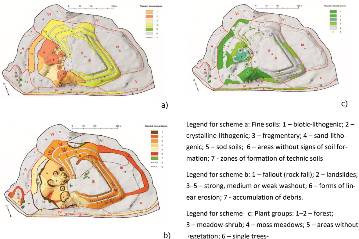
**Fig. 4.** Features of the formation and development of post-mining geosystems within the limits of the rock dump of the “Vizeyska” mine: a) soil formation; b) relief-making processes; c) formation of vegetation cover.
