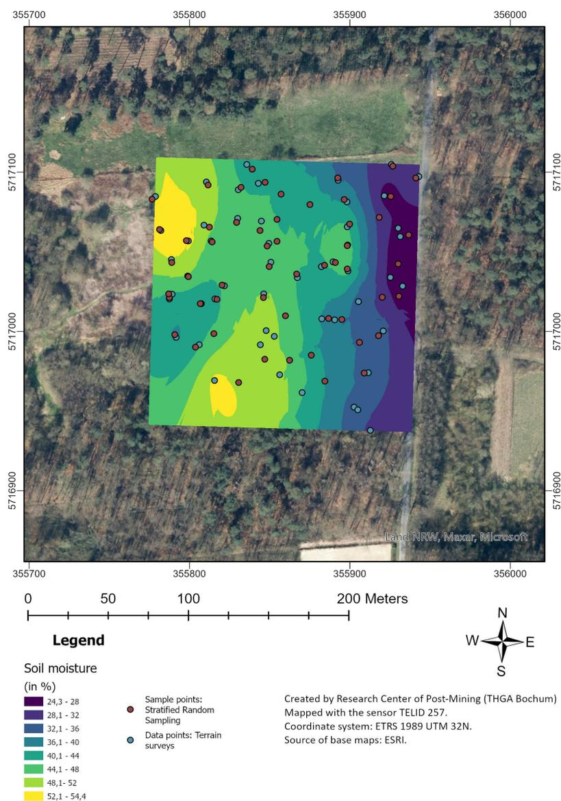
**Fig. 9.** Interpolation result using the SSUS-Method. For further description see text (Graphic: Marcin Pawlik, Bernsdorf et al. 2023).
