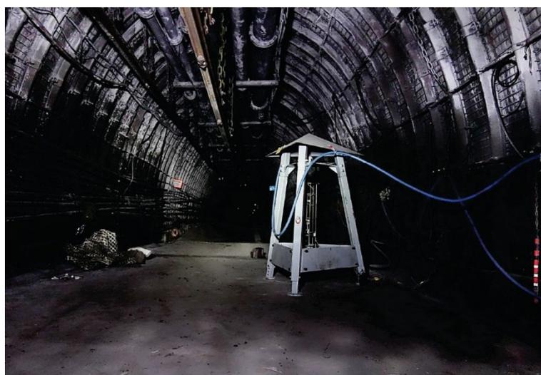
Fig. 3. Underground monitoring system for mine water rebound at the former coal mine Auguste Victoria (courtesy of RAG, Marin Schnieder, Martin Justa).
