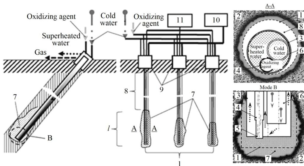
**Fig. 3.** Method of gasification of coal by autonomous boreholes: 1 – system of autonomous boreholes; 2 – coal seam; 3 – pipe recuperator; 4 – sleeve for supplying the oxidizer, 5 – nozzle; 6 – sleeve for supplying the heat-carrying agent, 7 – gasification zone; 8 – generator gas flow zone through the well; 9 – conductor; 10 – gas turbines; 11 – hydro-steam turbines
