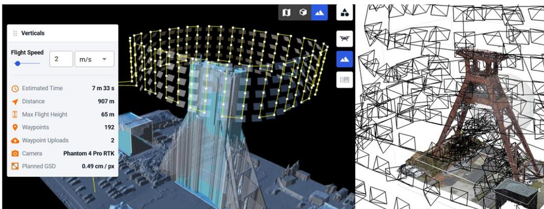
**Fig. 17.** Creation of high precision flight plans to perform the monitoring approach.
