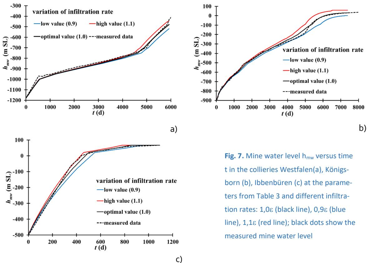
Fig. 7. Mine water level  $h_{mw}$  versus time  $t$  in the collieries Westfalen(a), Königsborn (b), Ibbenbüren (c) at the parameters from Table 3 and different infiltration rates: 1,0ε (black line), 0,9ε (blue line), 1,1ε (red line); black dots show the measured mine water level
