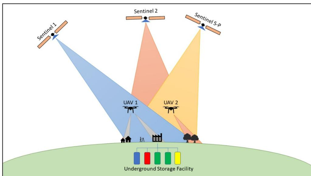
**Fig. 19.** Multi-layered, spatio-temporal geomonitoring of an underground storage facility developed in project KaMonSys (Haske et al. 2022).
