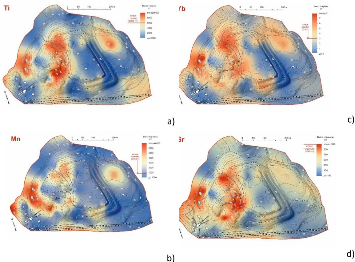
**Fig. 3.** The content of chemical elements in the lithological deposits of the rock dump of the “Vizeyska” mine: a) the content of titanium (Ti); b) manganese (Mn) content; c) ytterbium (Yb) content; d) content of strontium (Sr)
