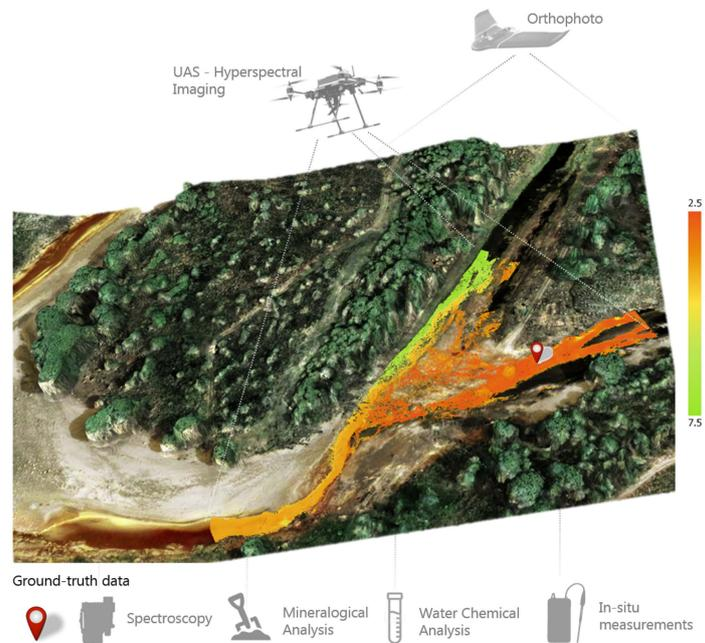
**Fig. 4.** 2.5D surface model representation of the AMD affected waters in southern Spain. Base layer are the combination of the orthophoto on top of the DSM and the produced regression-pH map for the river flow path (not drawn to scale). Modified from [31].
