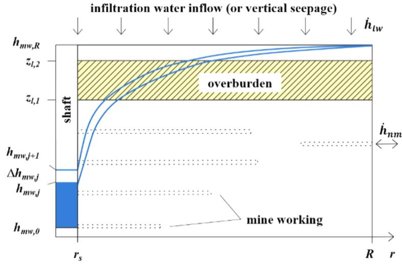
Fig. 1. Vertical cross-section of the flow domain
