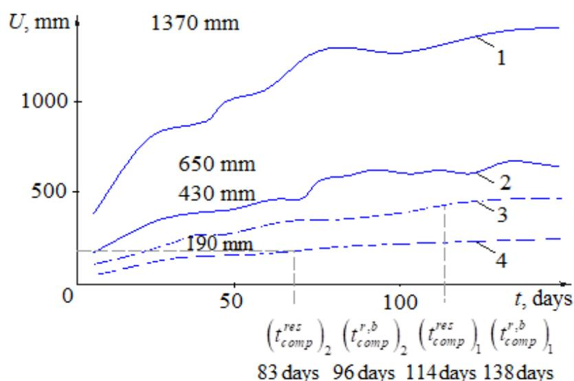
**Fig. 2.** Generalized dependences of the increase in displacements  $U$  of the mine working contour in time  $t$  of its supporting in the conditions of the Krasnoarmiisk coal-bearing region: 1 –  $\frac{H}{R} = 40$  m/MPa; 2 –  $\frac{H}{R} = 20$  m/MPa; —  $U^{r,b}(t)$ ; - - -  $U^{res}(t)$
