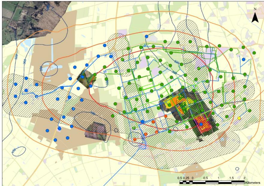
**Fig. 20.** The interactive GIS in the KaMonSys project. As an example, layers with information on pipelines, boreholes, caverns, land use, groundwater distances, ground subsidence, and geological faults are shown together with analyses of multispectral UAV flights (RGB, thermal infrared, NDVI).
