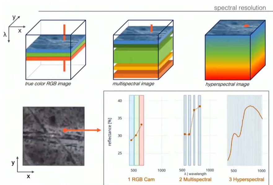
**Fig. 2.** Schematic examples on different levels of dimensionality of spectral data with  $x$ ,  $y$ ,  $\lambda$  being  $x$  and  $y$  the spatial and  $\lambda$  the spectral (modified from [9]).
