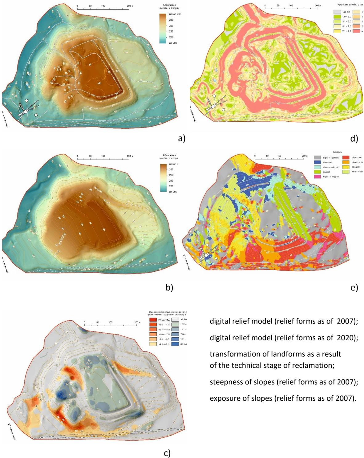
Fig. 1. Transformation of post-mining geosystems of the rock dump of the "Vizeyska" mine
