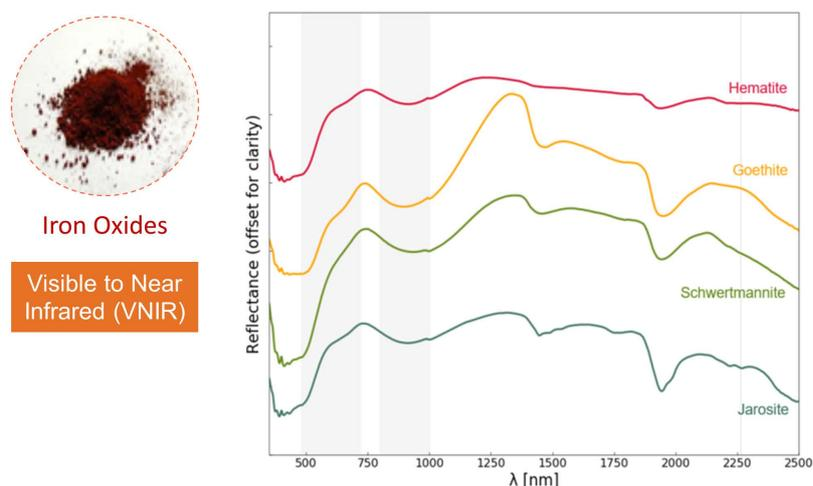
**Fig. 3.** Spectral curves for the main secondary iron-minerals typically of AMD (hematite, goethite, jarosite and schwertmannite), indicating prominent absorption features of each, using the spectral library of Crowley et al. (20).
