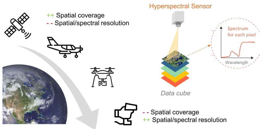
**Fig. 1.** Downscaling (multi-scale) scheme for hyperspectral sensing from high spatial cover age of satellite based sensors to high spectral resolution of drone-borne/terrestrial sensors and hyperspectral data cube scanning general concept. Source: THGA
