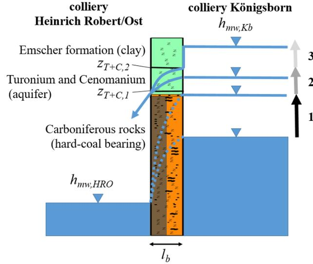
**Fig. 6.** Sketch to calculate water flow through the low-permeable barrier between two mines. 1, 2, 3 are the water levels in the flooded mine and ground water heads in the low-permeable barrier. Notations see in text
