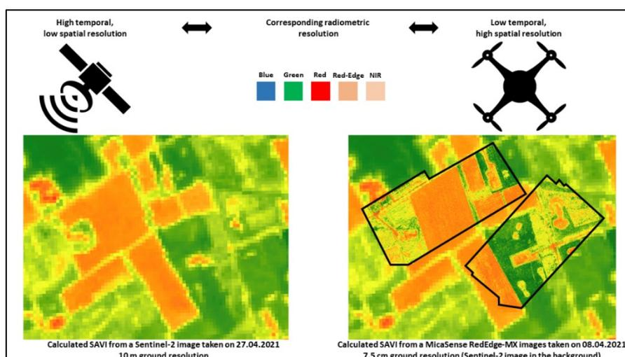
**Fig. 21.** Comparison between the spatial, temporal and spectral resolution of the Sentinel-2 satellite and a UAV-based MicaSense RedEdge-MX camera.
