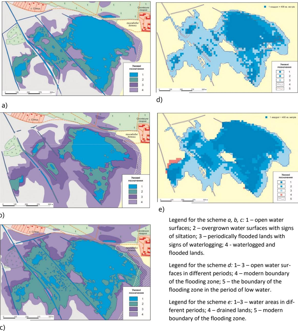
**Fig. 5.** Formation and development of post-mining geosystems within the subsidence mould of the earth's surface of the "Vizeyska" and "Nadia" mines (fragment of the map diagram): a) as of April 20, 2009; b) as of August 26, 2012; c) as of March 29, 2014; d) mosaic formation of open water surfaces; e) comparative mosaic dynamics of flooding of natural and economic systems.
