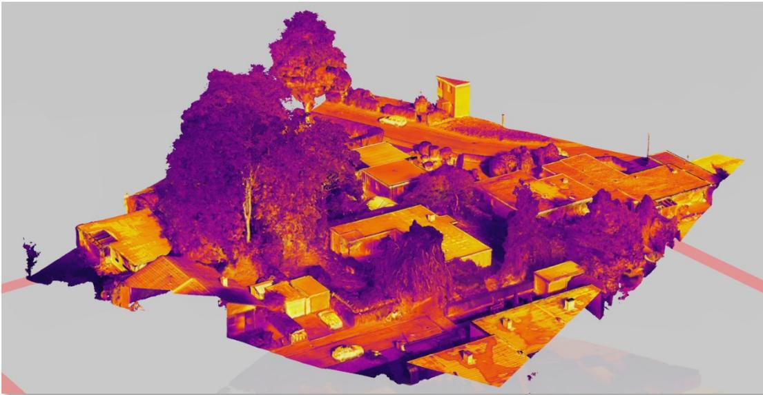
**Fig. 16.** 3D model based on an RGB orthophoto which “wears” a thermal image cover. Hoeschteel house, Dortmund (Drone flight Bodo Bernsdorf, modelling Benjamin Haske, FZN Bochum).
