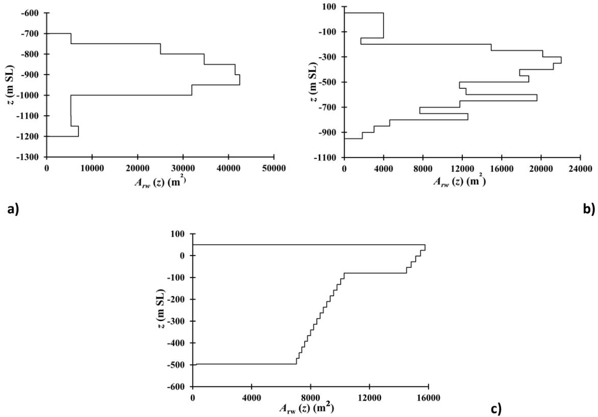
**Fig. 5.** Vertical distribution of the residual volume of underground workings expressed as the surface of a horizontal cross-section of the mine workings  $A_{rw}(z)$ : a) colliery Westfalen, b) colliery Königsborn, and 3) colliery Ibbenbüren (Westfeld)
