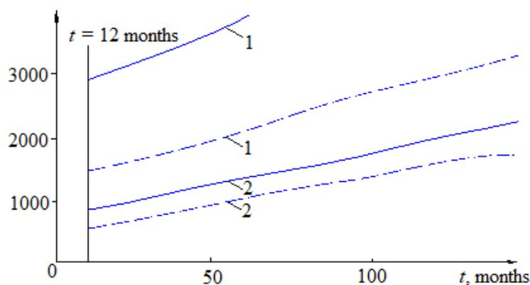
**Fig. 3.** Generalized dependences of growing displacements  $U$  of the mine working contour in time  $t$  of its supporting in the Western Donbas conditions with the undamping creep deformations of the lithotypes in the adjacent mass (the graphs are constructed taking into account periodic bottom ripping):
