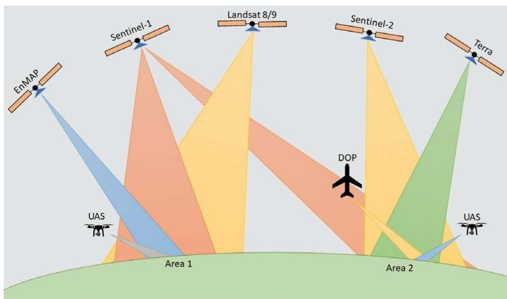
**Fig. 6.** Application of freely available remote sensing data, digital orthophotos (DOPs) and detailed UAS flights for the geomonitoring of target survey areas
