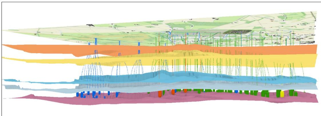
**Fig. 18.** Reused salt caverns for the storage of gaseous and liquid energy sources in northern Germany. Layers: Orange = Upper Bunter sandstone, Yellow = Dethfurt sandstone, Dark blue = Zechstein, Light blue = Werra rock salt, Purple = Lower Werra anhydrite. Caverns & Boreholes: Red = oil, Green = natural gas, Yellow = Red = oil, Green = natural gas, Yellow = helium, Blue = brine (Haske et al 2022).
