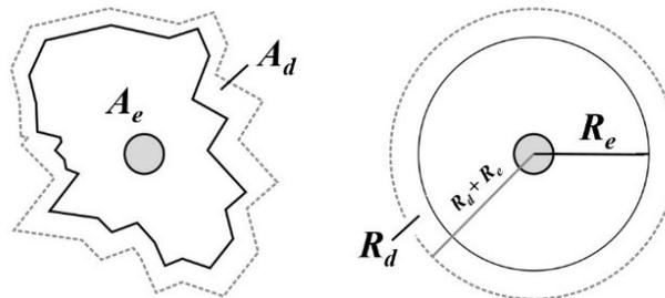
**Fig. 3.** Conversion of the real area of drainage influence (left) into the model-confirming shape (right)
