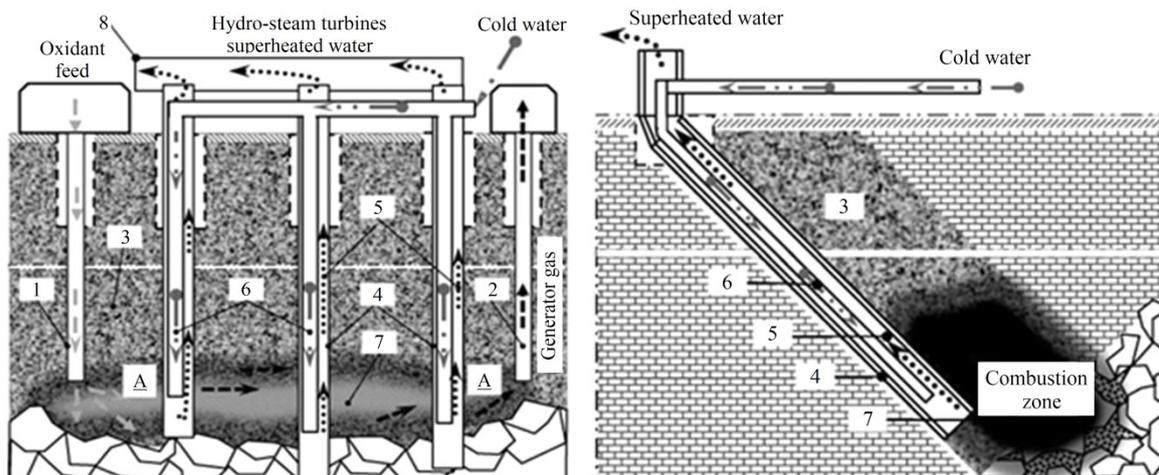
**Fig. 2.** Scheme of implementation of the method of thermal energy utilization for inclined seams: 1,2 – air input and productive boreholes; 3 – coal seam; 4 – heat removal boreholes; 5 – pipe sleeve; 6 – feed sleeve; 7 – seam gasification zone; 8 – hydro-steam turbines
