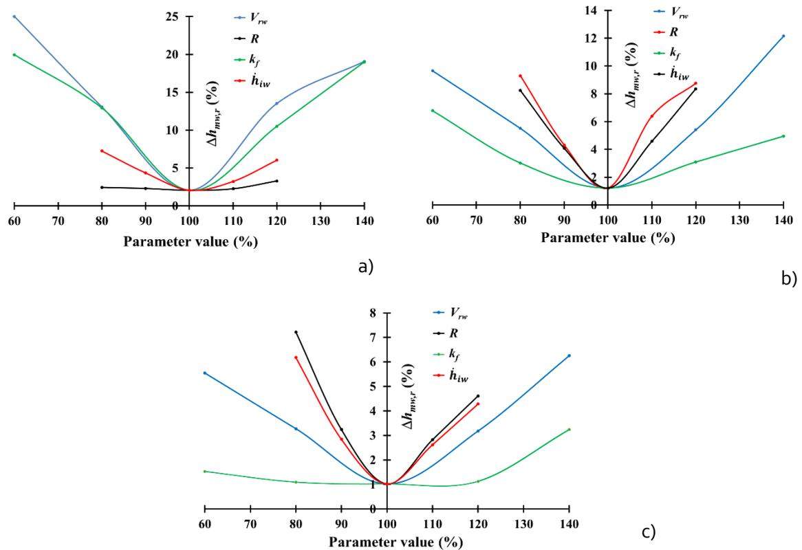
**Fig. 8.** Relative deviation  $\Delta h_{mw,r}$  between calculated and measured mine water level (Eq. 21) versus change of input parameters for the collieries Westfalen (a), Königsborn(b), Ibbenbüren (c)
