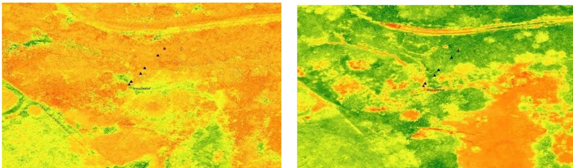
**Fig. 6.** “Green NDVI” derived from a RGB sensor of a DJI Mavic Air drone from February (left) and May 2021 (right). Red values indicate not yet developed vegetation, water areas and artificial landscape elements, green values healthy vegetation. The usual phenological development between the two months in the images can be seen (Bernsdorf et al 2022).
