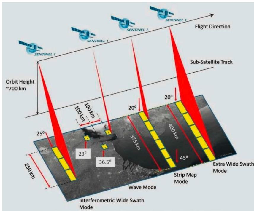
Fig. 2. Schematic representation of different recording methods and swath widths in satellite remote sensing using Sentinel 1 as an example [6]
