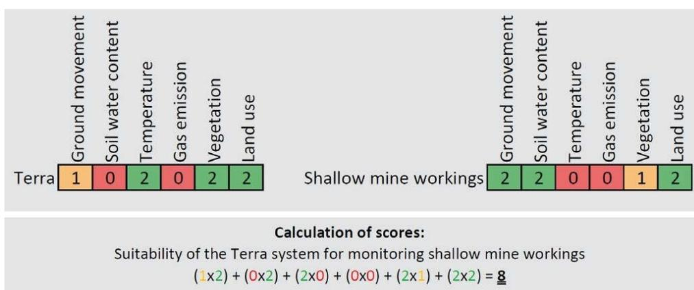
Fig. 4. Case example for calculating the suitability of a remote sensing system for monitoring a mining element
