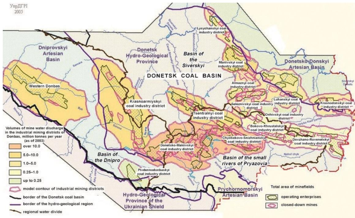
Fig. 1. Map of Donbas river basins: surface water resources and mine-water discharge
