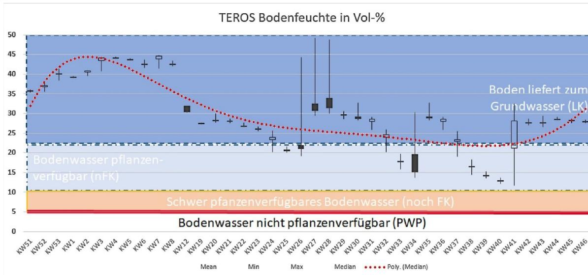
**Fig. 7.** Overlay of the soil moisture measurement data at Boye headwaters with the soil-physical characteristic values of the pF curve (Bernsdorf et al 2022).
