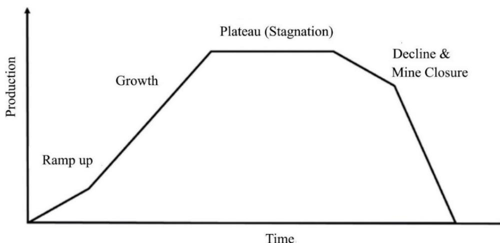
Fig. 1. The life cycle model for mining [6].
