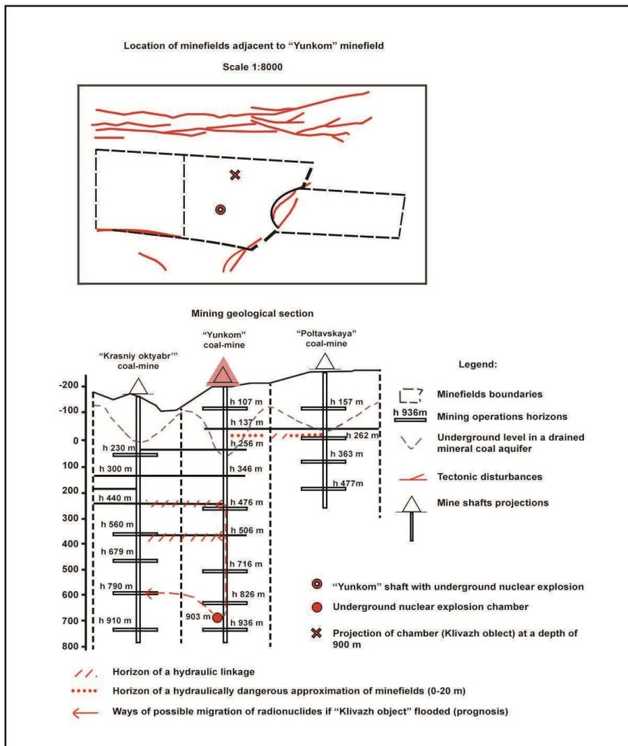
Fig. 4. The Yunkom mine area: adjacent minefields and a geological section
