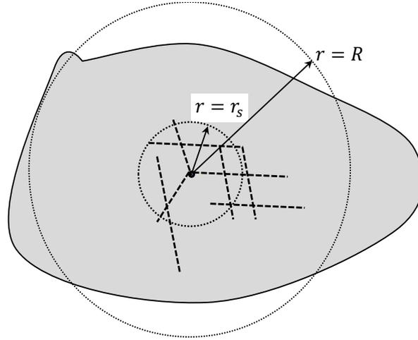
Fig. 2. Approximation of flow domain boundaries. Bold lines are real boundaries, a point is a shaft, dot lines are the circle approximation of outer and inner boundaries, and dash lines are the contours of underground workings
